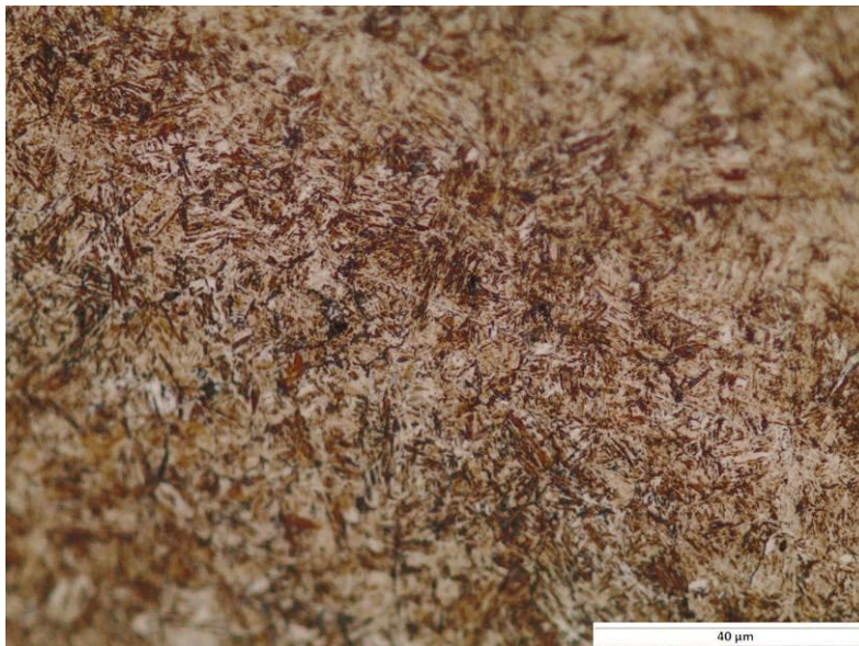
Figure 7: Martensitic microstructure of steel SAE 1045, after tempering heat treatment with water cooling and tempering (500x).
